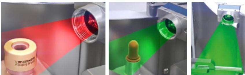
Through dedicated vision systems, it can be possible to check the entire quality of each component before the assembly. Only parts in compliance with costumer's quality standard will be feeded and assembled.
